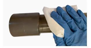
**Step 7** – Wipe off excess cement from the outside of the joint. Joint drying time will vary due to fit, amount of solvent cement applied, ambient temperature & working pressure. See below for detailed information.
