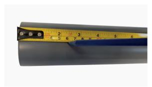
Measurement "b" should be used to check that the pipe is fully inserted into the socket after assembly.
