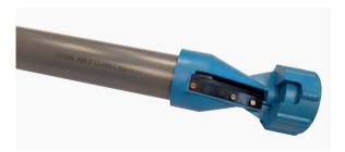
**Step 2** – Chamfer the pipe, approximately 3mm x 45°. This prevents the solvent cement layer being scraped from the surface of the fitting when the joint is assembled.
