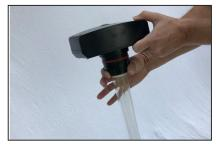
**Step 4 -** Remove the fixing-nut on the quartz glass tube .
