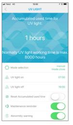
23. Accumulated time indicate time for change, Timer, Reset time when replacing bulb and get alerts and notifications.
