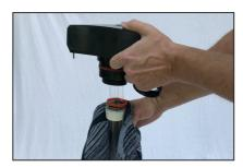
**Step 5 -** Pull out the quartz glass tube - then you can pull out and replace the UV lamp.
