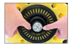
**Step 6 -** Now the filter sponges can be removed. The plastic holders in the middle of the sponges are easy to remove. Carefully dismount the small connections that hold the parts together.
