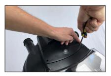
**Step 1 -** Unscrew the four screws under the rubber plugs on the lid of the UV-unit.
