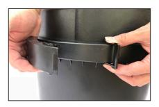
**Step 1** - Remove the protective cap and then open the large clamp on the cannister.
